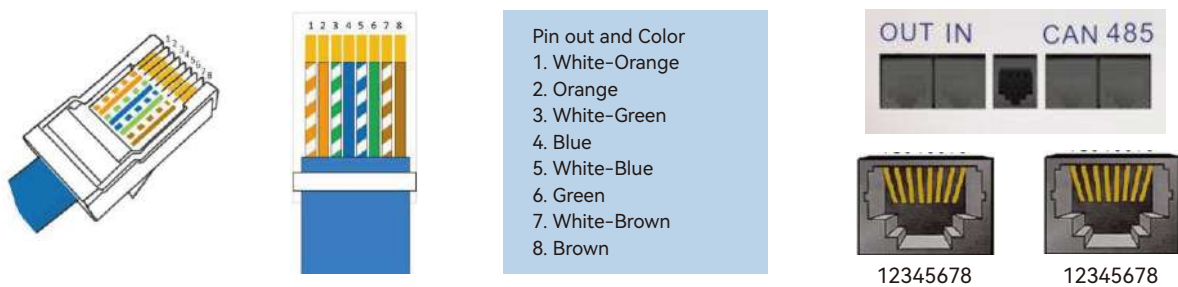
Figure 2-2 CAN, RS485, OUT, IN interface definition
