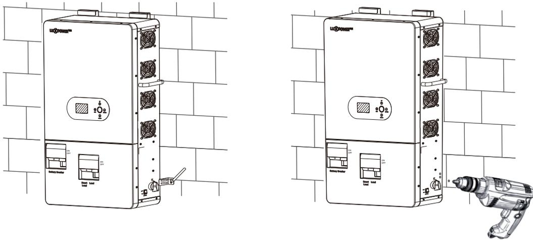
**Step 6.** Insert the expansion screws through the right-angle bracket into the drilled holes and secure them with M5 screws.
