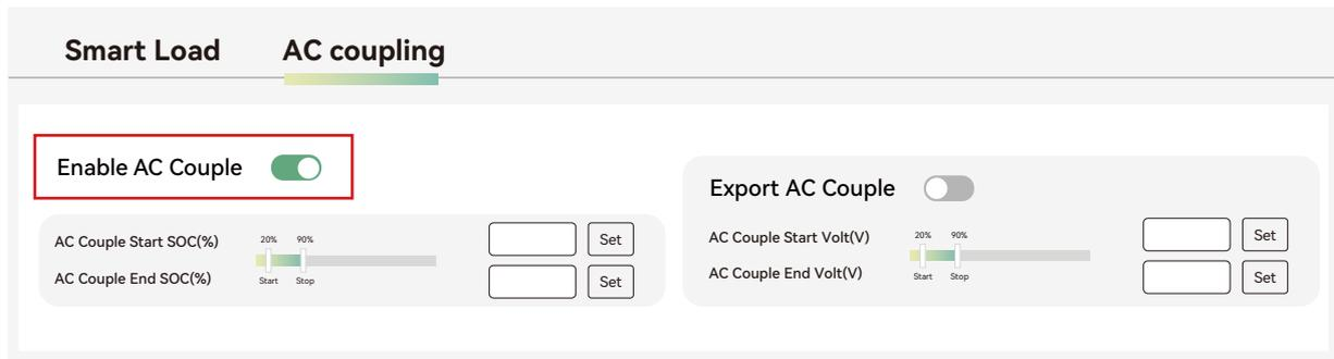
When on-grid and export to grid are enabled, the AC-coupled inverter will always be on, selling any extra power back to the grid. Ensure you are permitted to sell power to your utility provider when using AC-coupled PV arrays on-grid.
