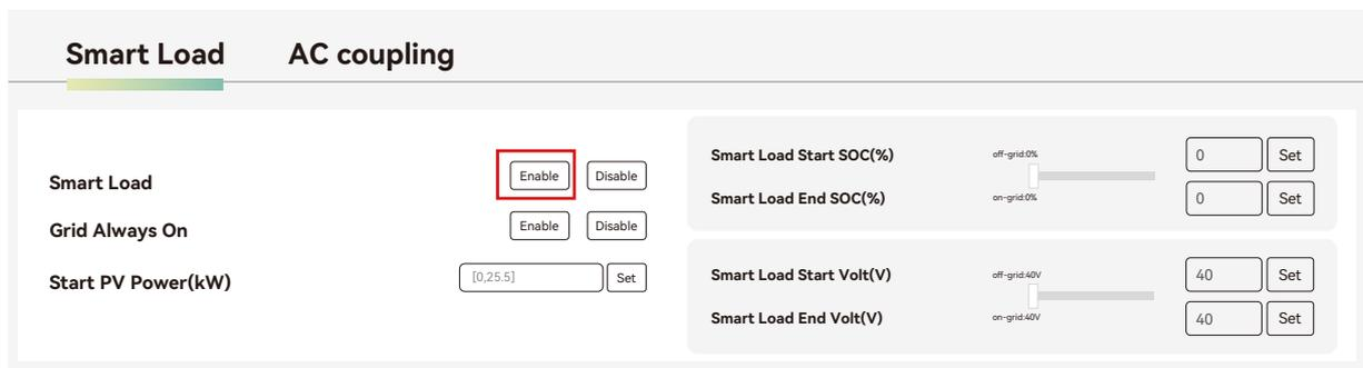
Enable “Grid always on”: When connected to the grid, the smart load remains continuously connected.
