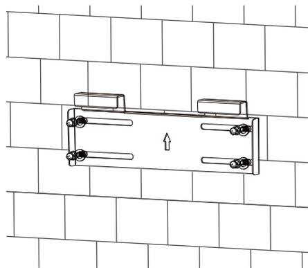
**Step 4.** Lift the inverter and secure it onto the wall mount.
