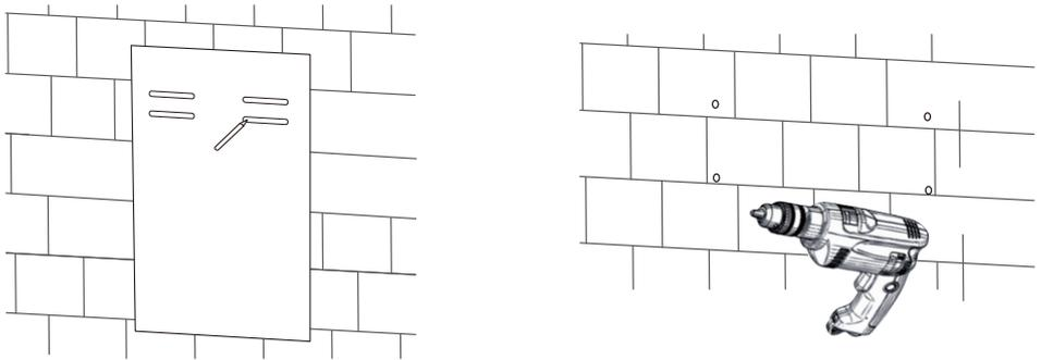
**Step 2.** Remove the positioning plate and insert M8 expansion screws into the holes.
