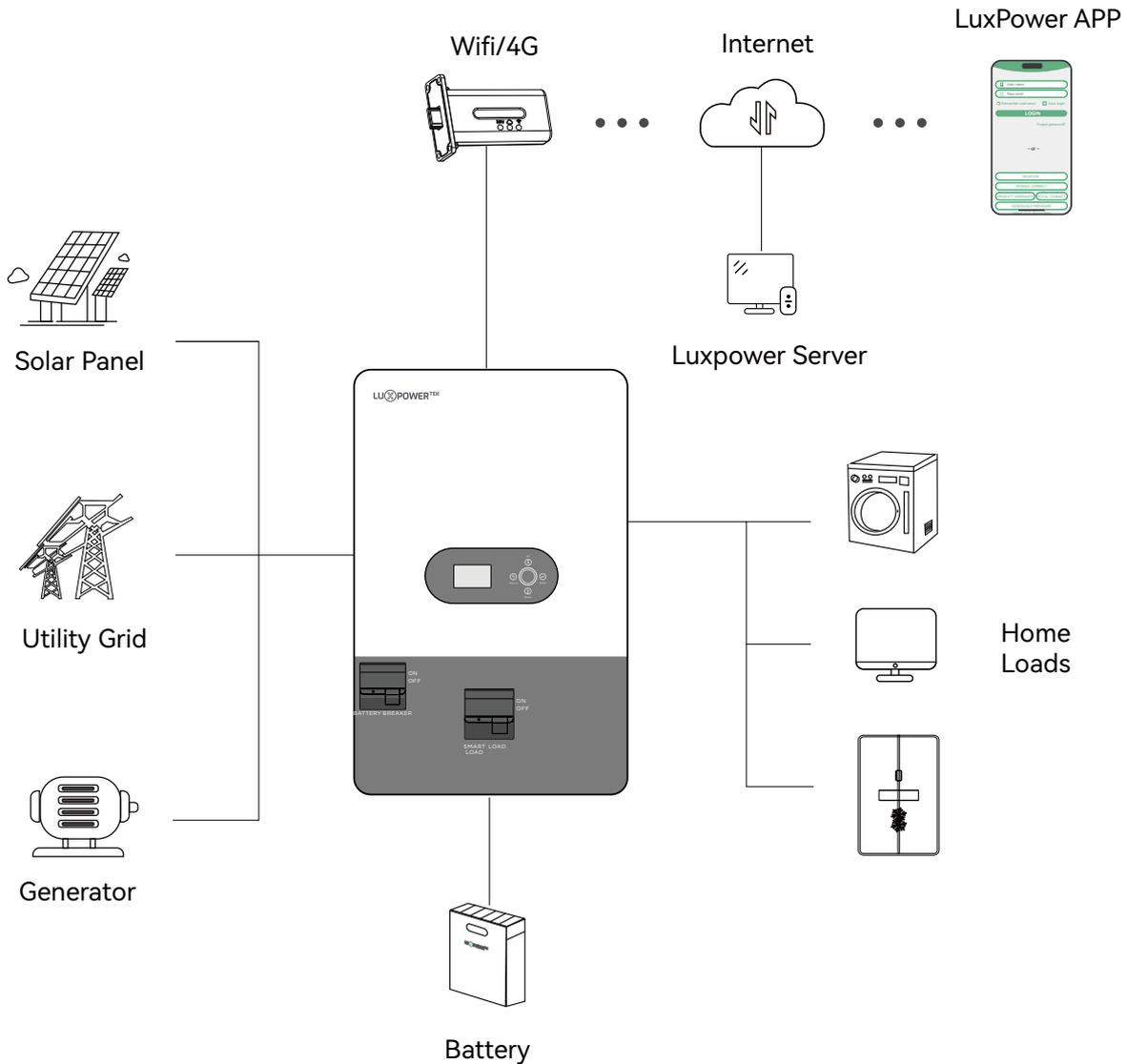
SNA series is a multifunctional, high frequency pure sine wave Offgrid inverter solar inverter, features:
