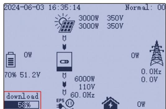
If the system displays the icon in the red box. Indicates that the AC input port is connected to the power grid.
