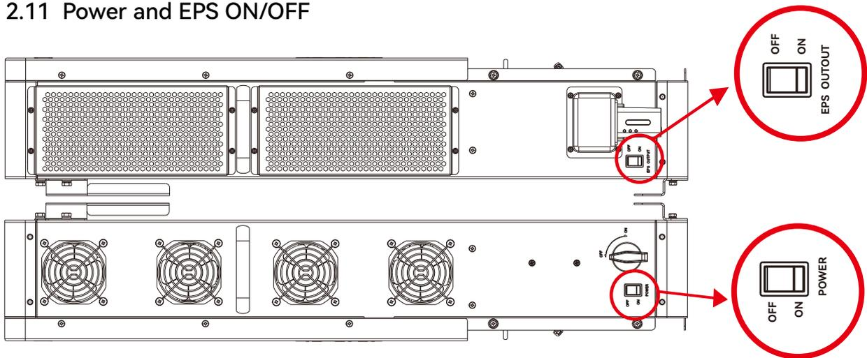
1. Power Switch: Control power supply for the unit
