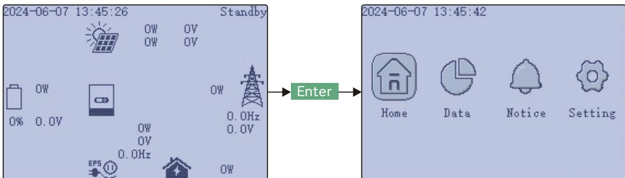
Using the UP and DOWN buttons, select the desired function, then press ENTER to enter. Press Return to return to the previous level. The options include Home for the main page, Data for operational data, Notice for fault and warning information, and Setting for configuration settings.
