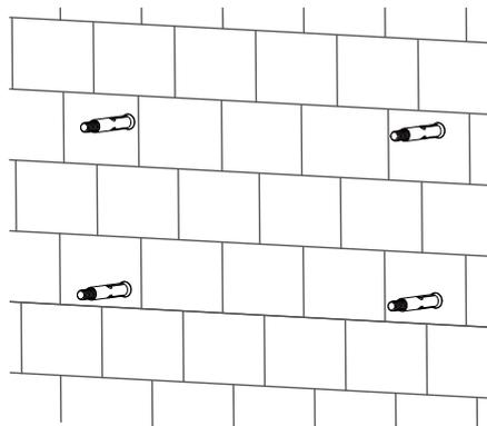
**Step 3.** Attach the wall mount to the expansion screws and secure it (pay attention to the direction of the arrows on the wall mount).
