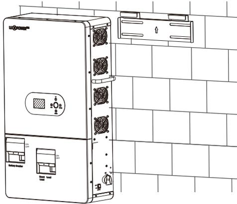
**Step 5.** Take out the right-angle fixing clip, find the holes on the inverter (located at the bottom, one on each side), and drill holes on the wall based on the positions of the right-angle clip holes.
