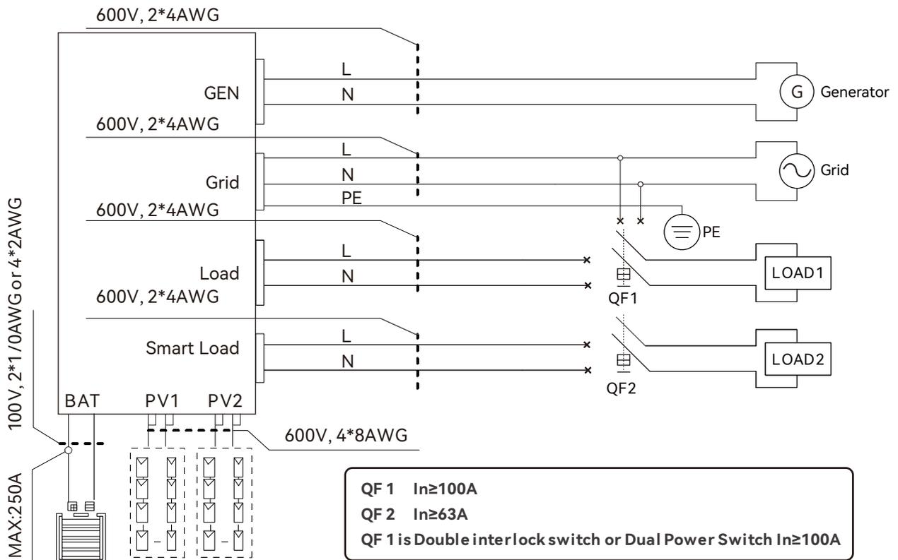
Please prepare the breakers and cables in advanced before installation.
