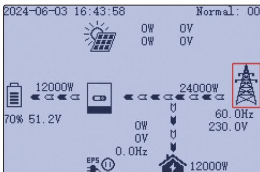
When the icon in the red box is displayed, it indicates that the AC input port is connected to a generator.
