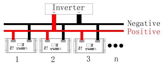
Wiring Diagram of Battery Pack in Parallel (Figure 2)
