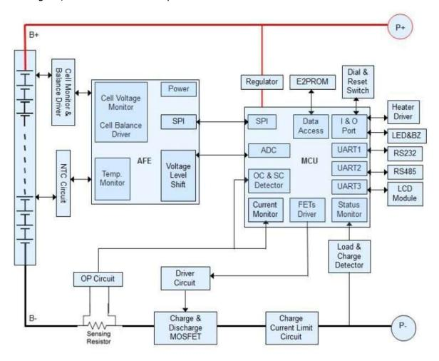
Fig1 Battery Block Diagram
