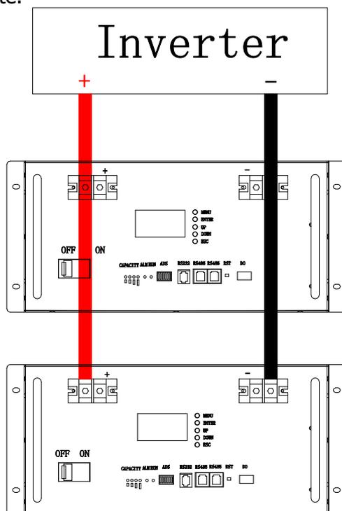
**Wiring Diagram of Battery Pack in Parallel (Figure 1)**
