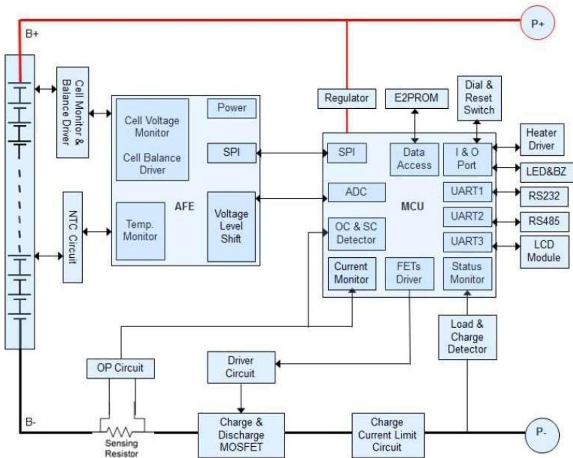
**Fig1 Battery Block Diagram**
