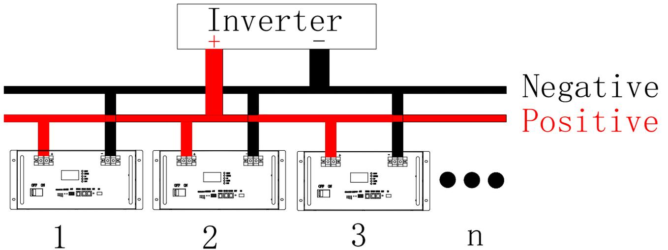
**Wiring Diagram of Battery Pack in Parallel (Figure 2)**
